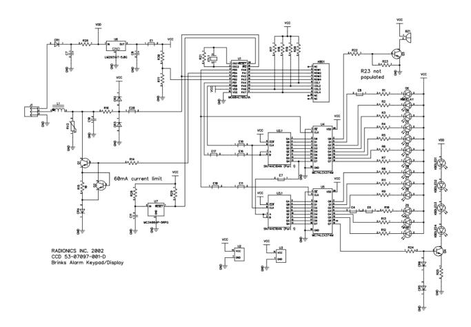
The main issue here was that it used a Motorola MC68HC705 processor chip and I didn't have any development tools for it, so I designed a small adapter board that would allow me to use a PIC16F15244 processor instead.
