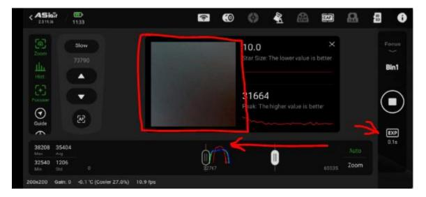
By adjusting the exposure time down (from 0.2 seconds -> 0.1 second) you can see that the Histogram has moved more to the middle of the range and the image is no longer washed out – although is still seriously out of focus.
