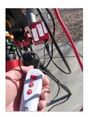
The benefit if this is that it works almost like the original focus knob allowing you to easily adjust the focus up or down in a more natural way then repeatedly tapping the app touch screen buttons.
