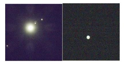
What happens then is that, after the mount has moved to point to Jupiter, it tries to center, but constantly fails with an error message like: "385 stars detected" ... "unable to center" ... "retrying." The only way to get this to stop is to turn off the "GoTo Auto-Center" option (see above) Mount setting – however this leaves your target not quite in the center of the camera.
