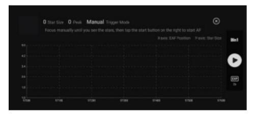
Press the big '>' play button and the auto focus will adjust the focus up and down until the focus is exact as possible.
