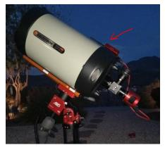
If your ASIAir ends up being mounted on your telescope (which is very common to facilitate the cabling) it will move around as you move from target to target, or simply track a targets movement over time. When this happens, it is important that you remember to manually re-orient the antenna so that it is pointing either up or down. If you fail to do this you may encounter cases where the ASIAir drops off the WiFi network and loses communication with the app.
