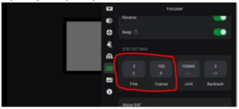
You may have to do this several times. When you are way out of focus, your Fine/Coarse settings will need to start with large numbers such as 200/1000 (which approximates the accuracy of turning the focus knob with your hand.) As you get the object more in focus you will want to use smaller numbers like 20/100
