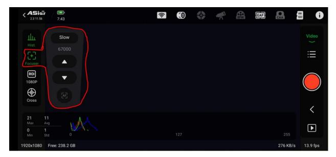
However, this button is almost useless (at least in Station Mode – I haven't tried it in Direct Mode) because of the huge lag delay (often around 30 seconds) between you pressing the 'up' or 'down' buttons and the focus actually changing while the video is running.
