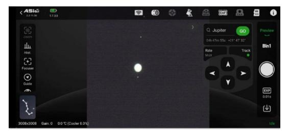
As can be seen Jupiter is a little to the left of the center, so you can probably just go to Video mode. If Jupiter were way off center, you would need to get it in the center first by using the mount movement arrow keys. Typically, the mount movement arrow keys will have the following effect on the target:
