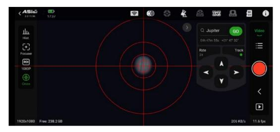
Now start the EAF to move to the Barlow focus point of 67000 (or wherever you previously determined the Barlow rough focus to be.) As it slowly moves Jupiter will get out of focus and start to move around out of the cross-hair center – this is because the mirror is moving of course. Be alert and use the mount movement arrow keys in 2x rate to keep the ever blurrier circle roughly in the center.
