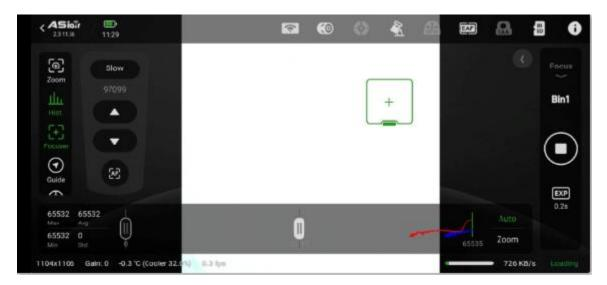
Even though you are still pointing at the same target (radio tower) the Barlow has completely altered the light path and you need to re-adjust everything. The first thing to note is that Histogram which is now showing a signal clipped on the right side indicating that the image is over-exposed.
