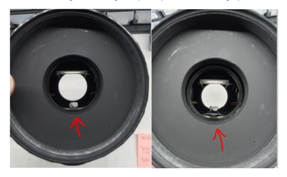
Note how much more of the prism is exposed to the light path in right 'high' configuration. The low configuration is intended for cases where the S52 Flip Mirror light path is chosen.
