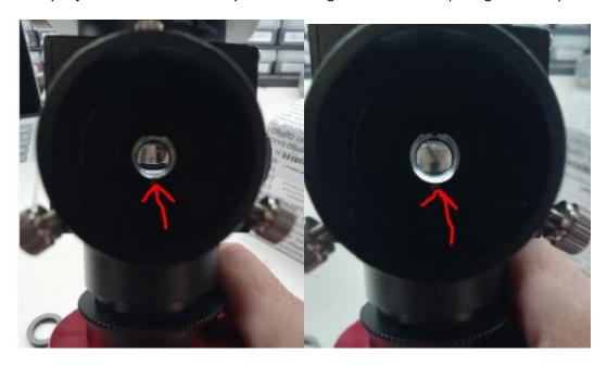
Your prism is now correctly aligned in the light path.
