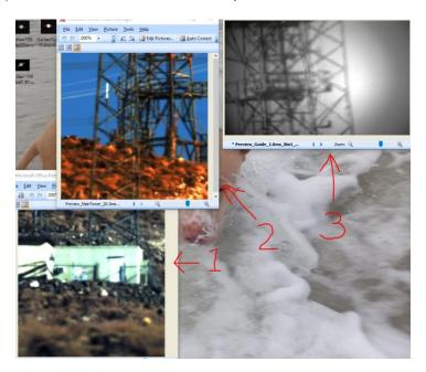
Note that (3) is flipped horizontally from the true image (but correct vertically.) Rotating the guide camera 180 degrees results in an image that is correct horizontally (but flipped vertically.)
