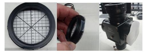
Then you can accurately do the alignment while looking up the OAG tube as shown below.
