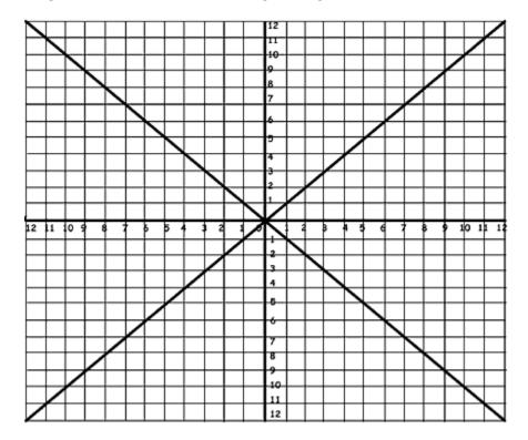
Take a graticule (example above) and cut it out so it fits over the end of the appropriately sized light path tube extension (see below where I used an M48-SCT adapter.)
