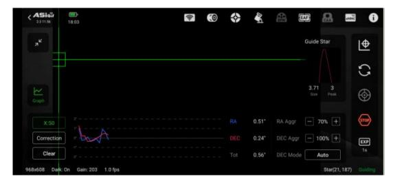
Initially there may be some 'jumping around' of the guiding system until everything stabilizes. Over time this will stabilize and the graph will smooth out and you can see how close the guidance system is keeping your target (the smaller the deviations the better.)
