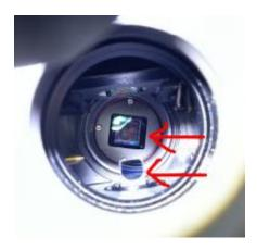
Although much less critical, you should also make sure the prism is not obscured by the flip mirror when the mirror is in the down position. This is less critical because it doesn't really matter if guiding is working when using the eyepiece – although it may be annoying to keep getting messages from the controller that guiding stopped.
