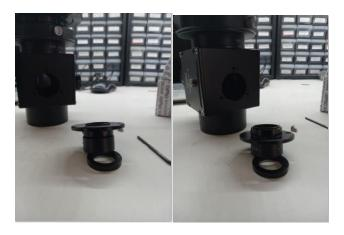
Using the optional spacer would make each of the scenarios so the mirror is even lower. Below you can see how each of these configurations changes the prism's position in the M48 light path.
