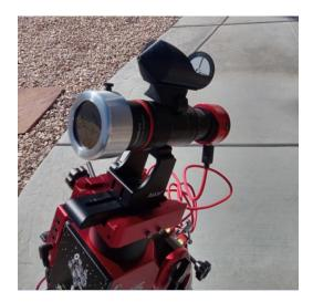
First of all, you will need the <u>BuckeyeStargazer Sun Finder</u> (mounted on top of the telescope above.) It seems odd to need a tool to "find" the sun, but since you can't look at the sun, the only way to align the scope is to use the suns image on backscreen cross hairs.
