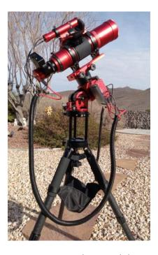
This really helps when the telescope is pointing straight up and the camera tends to hit the tripod legs as it rotates. Needless to say, the pier raises the center of gravity and makes the whole assembly less stable, so you should consider adding extra weight to the tripod (in the hanging bag below) to make it more stable.
