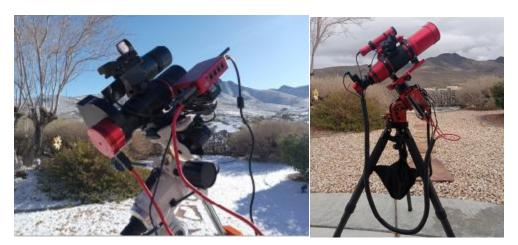
I also had to move where the ASIAir was mounted as it and the cables coming out of it would hit the tripod in extreme cases. Additionally, I wanted the ASIAir mounted to the tripod so that I wouldn't have to move it between telescope mounts when switching telescopes for different targets.
