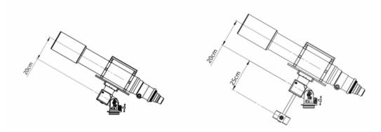
Additionally, for large SCTs (like my C11) the scope center axis is about 12" (30.48cm) above the AM5 center of rotation so some portion of the AM5 load capacity is lost. So perhaps 1/3 of the load capacity is lost (if the relationship is linear) giving it a load capacity of only 29lbs, and explaining why some extra counterweight is needed in this application.
