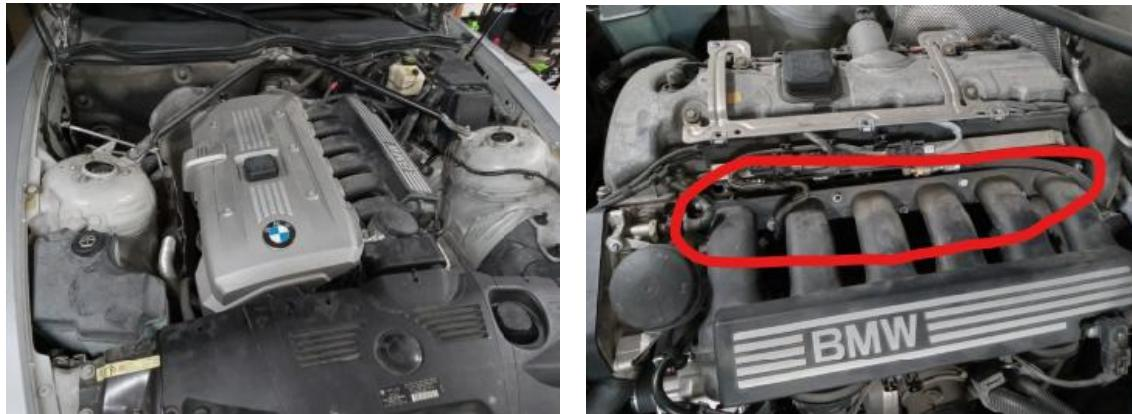
There are various hoses and cables that also need to be disconnected so that you pull the manifold away from the engine – these are not documented here.
