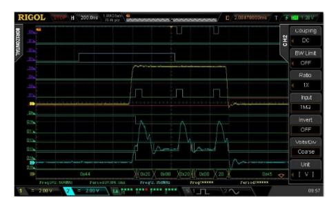
The D5 data line looks horrible and has a very slow rise time compared to the ADSTB above it. It is for this reason that the latch is latching a value of '0' for A13, instead of '1' which would be registered if the D5 data line had a better rise time and cleaner signal.
