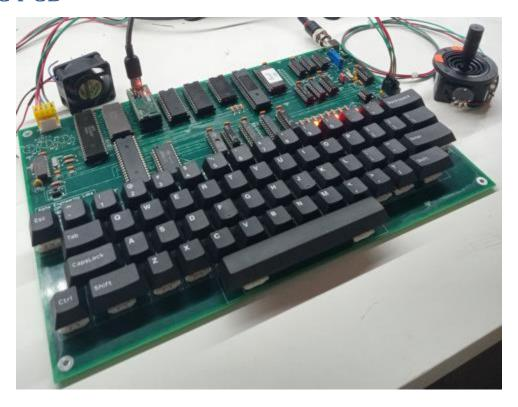
The rev C PCB was generated after all of the preceding debug was completed – to resolve the issues found as well as to add a joystick interface so that simple video games could be programmed.
