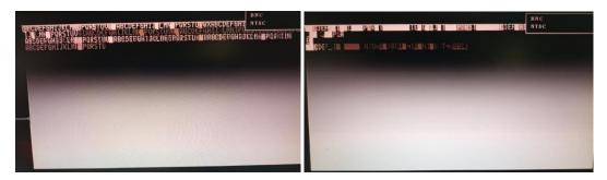
This seems to contradict the spec, as I would have expected the results to be "better" in the right image (not worse.) But it does prove that altering the RAM access times does indeed have an effect on the DMA data transferred.
