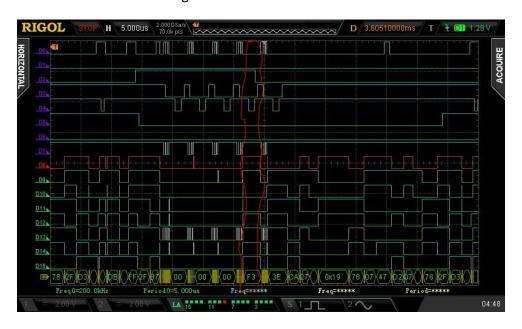
I was able to verify that the video interrupt logic is working properly (see below – yellow scope line is DMA chip select and red circled pulses are IOWR active with DMA CS.) You will have to take my word but if you expand the view, you will see that the data written out in these 5 writes is: 0x01, 0x06, 0x20, 0x7f, 0x87.
