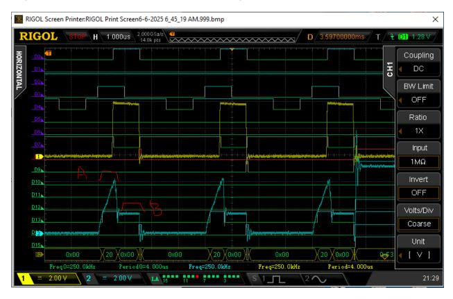
You can see in section 'A' adding the pull-up resistor "fixed" the problem by pulling up the floating data bus so that the value can be correctly read by the 8212 on the rising edge of ASTB. You can then see in section 'B' where the DMA actually starts driving the data bus (in this case D5) to a value of '1' so that it is stable before the falling edge of ASTB.
