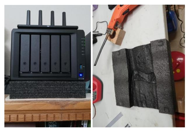
IMPORTANT – you must cut out an air channel in the foam (as shown in the image on the right above) so that the SSD cooling slots on the bottom of the chassis can receive air flow. Failure to do this results in the SSD and logic board running about 25 degrees fahrenheit hotter than normal.
