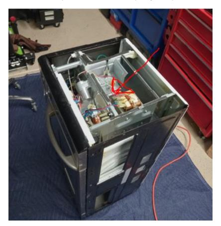
You will need to transfer the metal wing and the black sensor from the old magnetron to the new one.
