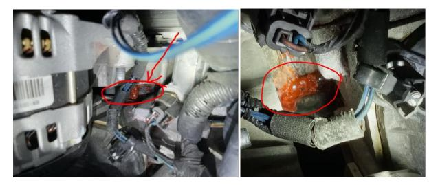
There were other smaller leaks on the upper left hand side of the timing belt cover (below left) and on the bottom of the timing belt cover (below right.)
