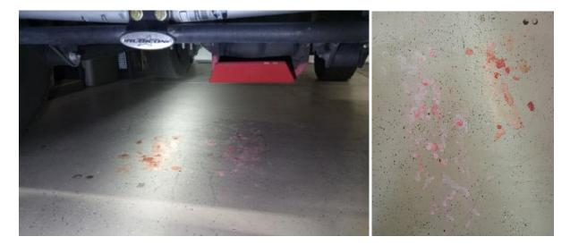
At first I thought this might be Freon because the trails appeared to come from the bottom of the compressor. However, after tracking it down further it turned out to be anti-freeze coming out from different points on the timing belt cover gasket as can be seen below in the upper right side of the timing belt cover.
