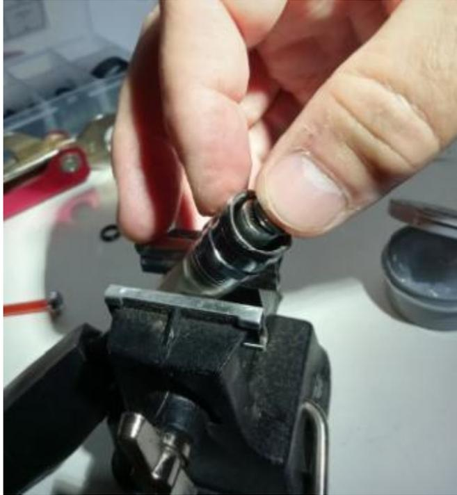
Complete by re-attaching the hose to the second stage regulator.
