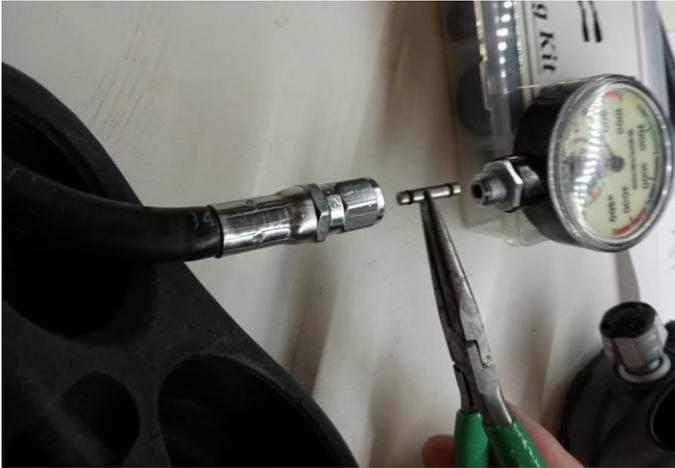
4. Pull the swivel pin out of the assembly (seen in pliers above.)
