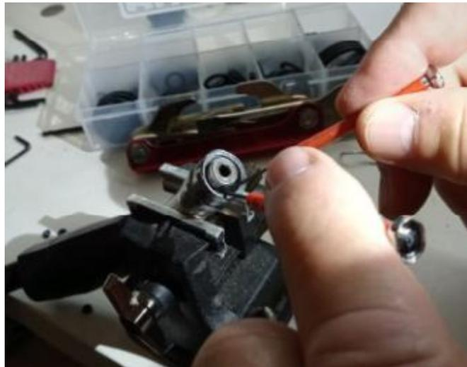
To insert the new o-ring, apply a thin film of silicone grease to an AS-012 (3/8") o-ring and slide it over the metal tip of the hose and gently roll it down into the o-ring groove.
