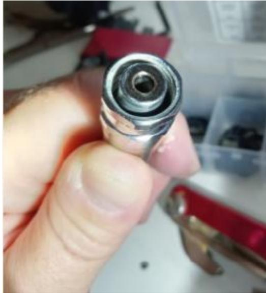
The fact that it is recessed makes it more difficult to get out, but getting it back in is easy. After trying various things (that didn't work) I found that a small vise and some 1mm jewelers screw drivers worked really well. The easiest way is to break the old o-ring with one of the screw drivers and then position both of the screw drivers in the break and push the broken o-ring out of the slot.
