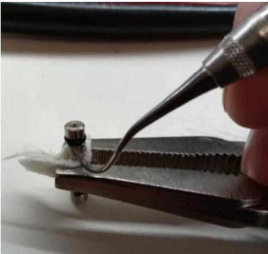
6. Lightly coat an AS-003 (1/16") o-ring with silicone grease. Do not forget this step as it makes it much easier to slide the o-ring over the pin!
