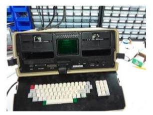
With the keyboard finally functional, I was able to proceed to try and get the computer to boot from the floppy drives.
