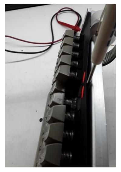
I then simply 'jammed' a screwdriver between the two layers of the membrane keyboard and twisted it around where the contact points for the two questionable switches were located.
