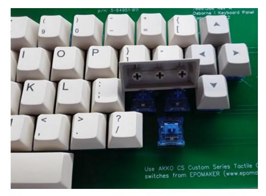
The first thing to do was to file down the 'Enter' keycap until it would fit between the other two keys. And then using a Dremel tool, remove the outside two posts of the 'Enter' keycap. The center post could stay as it passed harmlessly between the two switches.
