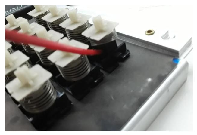
At first I couldn't figure out how to take the keys apart without breaking them. After reviewing some other comments on the internet it became clear that you just had to 'yank' the white plastic tops off. This worked fine and I was able to see 'inside' the switch, however I was not able to find any visible cause for the shorts.
