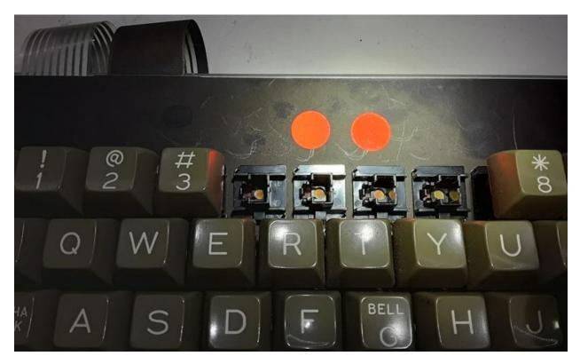
The difficulty in repairing this problem lay in the fact that the keyboard was not designed to be taken apart. Each of the plastic key housings had extrusions that when through holes in the keyboard chassis and had been 'melted' down to permanently attach them mechanically to the chassis.
