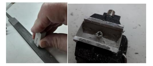
Then it was necessary to 'steal' two mounting points from other unused keycaps. This also was done using a Dremel tool.
