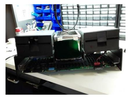
The drive head carriage was 'frozen' on the rails (see below – highlighted in yellow.) This caused the head to be unable to move from track to track and properly read the disk. This was a problem on both of the drives.
