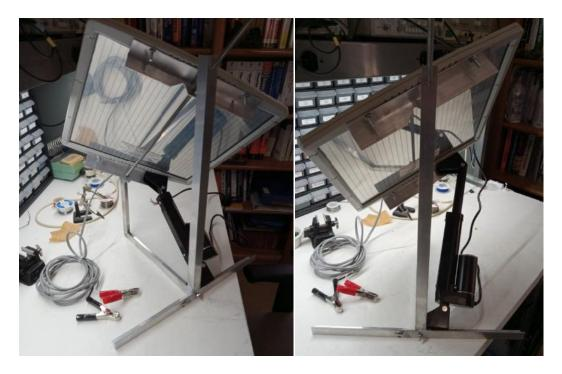
As can be seen above the finished bracket has a single linear actuator that allows the panel to rotate around its axis to follow the sun.
