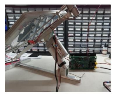
This bracket supports two actuators: (1) the linear actuator used to tilt the panel to change the inclination based on the season of the year, and (2) the angular actuator used to rotate the panel around its axis to follow the sun during the day.
