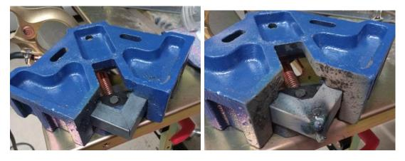
After a lot of grinding and polishing I was able to clean up the messy, but solid welds as shown below.
