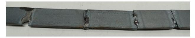
Welds front – after cleaning with wire wheel
