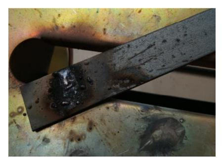
I then did a bunch of other welds (below left) and after turning the bar over I could observe that most of them penetrated pretty well (below right.) I did these all at 100A DC per the Miller weld calculator recommendation which said 110-165, but I can only get 100A using a 110VAC outlet.
