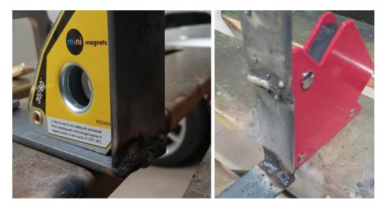
Note that the fixturing magnets (which were useless for TIG welding aluminum) are now coming in handy.
